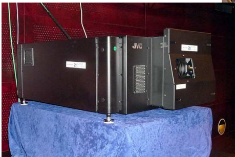
The SHV projector in place at the back of the cinema, and part of the 22.2 sound installation arranged around the projection screen
